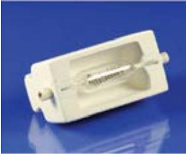
The OL 100 is a high-intensity standard consisting of a 1000-watt, DXW, tungsten-halogen lamp mounted in a slip-cast, fused silica reflector. The source has an effective radiating area of 3 x 5 cm. At a distance of 40 cm, the total irradiance is on the order of one solar constant (approx-
