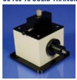
Utilized for performing spectral transmittance measurements of samples in solid form. Has a slide-in sample holder that accommodates both 1-inch by 1-inch, and 2-inch by 2-inch square samples, as well as 1-inch diameter and 2-inch diameter round samples. Samples can be up to ½-inch in thickness
