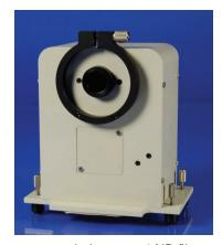
The OL 770-15Q-A Neutral Density (ND) Filter Wheel is an automated alternative to the OL 770-15Q Neutral Density Filter Holder, which requires manual insertion of the ND filters and selection of the corresponding filter coefficients in the OL 770 application. The OL 770-15Q-A contains 5 filter positions for
