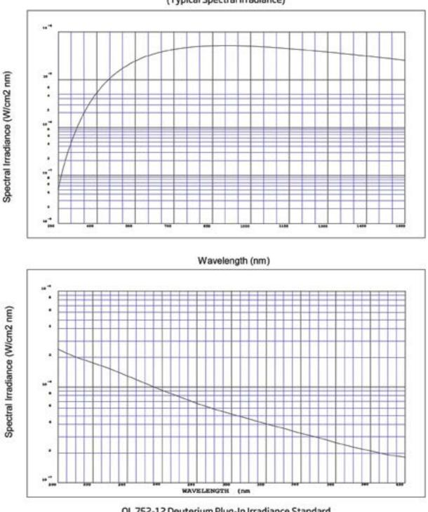
OL 752-10 Tungsten Plug-in Irradiance Standard (Typical Spectral Irradiance)
