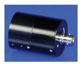
The OL 730-5A and OL 730-5C UV Enhanced Silicon Detectors are 1 cm<sup>2</sup> active area, high impedance, low capacitance, planar diffusion photodiodes. These detectors, which are sensitive over the wavelength range of 200 to 1100
