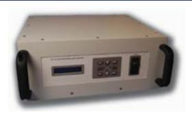
The OL 410 is a microprocessor-controlled, precision DC lamp source specifically designed to accurately operate tungsten filament lamp standards and calibration sources. The power output range is 150 watts for the OL 410-150, 200 watts for the OL 410-200, and 1000 watts for the OL 410-1000.
