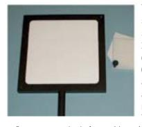
The Optronic Laboratories specular reflectance standards are available in 2 x 2 inch (OL 25RS-S) or circular 1-inch diameter (OL 10RS-S) sizes. These are front surface coated aluminum mirrors with a magnesium fluoride overcoat. They are used as specular
