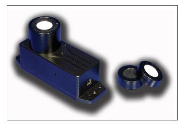
The OL 731 USB Smart Detector is a low-cost, flexible, programmable, compact radiometer-photometer that can easily be set up for specialized needs. A range of sensors and filters are available to tailor the spectral response to the application - specific requirements. A command set is provided to enable the creation of acquisition programs. As delivered, the OL 731 Series detectors can be operated by any computer with a USB connection.
