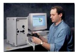
The Labsphere LED-1100 combines CIE Condition B for averaged LED intensity with a goniometer. Although it is advertised as a spectroradiometer, the CCD spectrograph is only used for chromaticity. A filtered photodiode is used for Condition B measurements and a raw photodiode is used for goniometric measurements. This is a cumbersome configuration that can yield significant errors and should be avoided. Other points to consider are:
