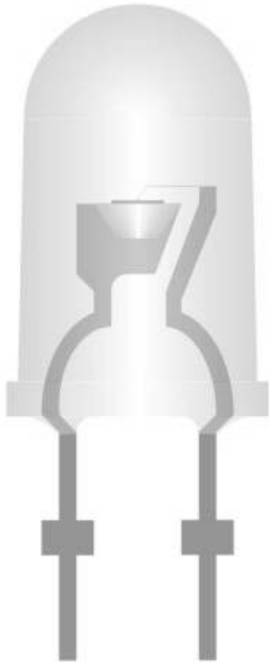
Fig. 1. A packaged LED comprises several complex structures in addition to the chip.
